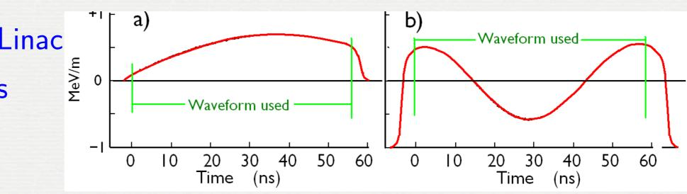
Pulse shape adjusted to maintain elliptical profile in longitudinal phase space.
