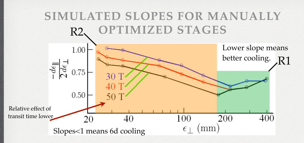
• Going to higher negative dE/dx slopes makes longitudinal heating worse.
